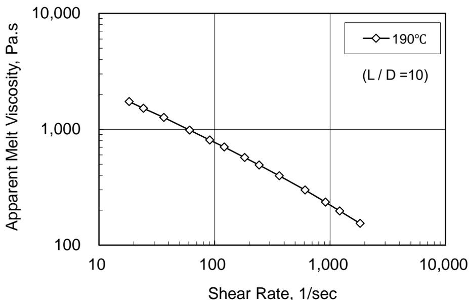
Fig. 1 Melt Viscosity of Soaresin™ RG100
