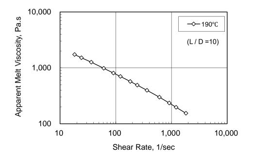
Fig. 1 Melt Viscosity of Soaresin™ RG100
